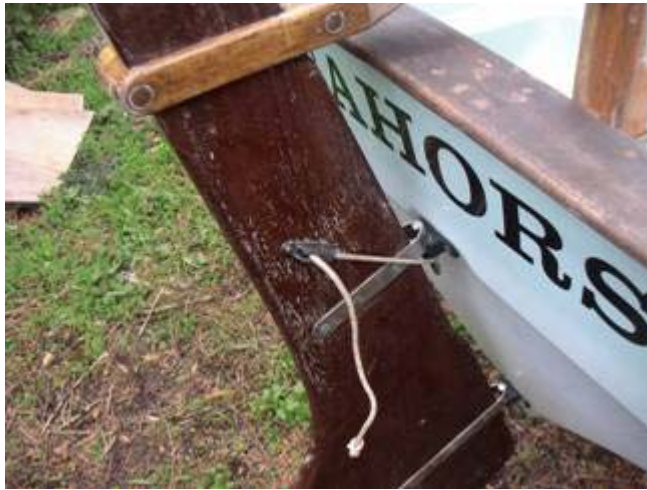
Fig. 1 Rudder retention line
