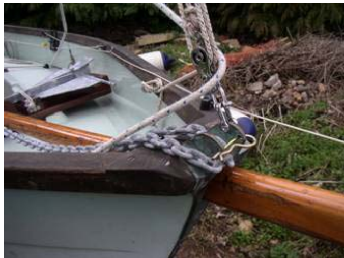
Fig. 7 R clip in the bow casting. The chain is spliced directly to octoplate anchorline, which allows it to run out below the clip. The cleating of the forestay tackle can be seen on the port gunwale.
