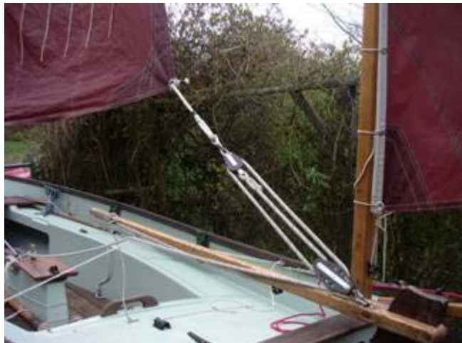
Fig. 5 Main sheet arrangement
